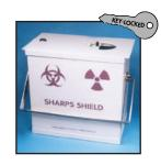
039-335 Sharps Container Shield Shield uses 039-341 Dimensions: 7.5" l x 12.5" w x 13" h (19 x 32 x 33 cm) I.D.: 6.875" l x 10.75" w x 12.5" h (17.5 x 27 x 32 cm) Lead Shielding: .125" thick (.32 cm) Security: Key-locked Finish: Powder coat Weight: 53 lb (24 kg)
