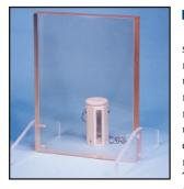
The Bench Top Shield for gamma radiation is constructed of 1.375" thick (35 mm) lead acrylic, providing the equivalent of 0.060" (1.5 mm) lead for shielding gamma radiation. Lead acrylic can be used with low-energy gamma emitters. Lead acrylic is not recommended for beta emitters. This lightweight, sturdy shield is ideal for use in hoods, on labo-
