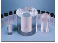
The Neck Phantom is designed to simulate a patient's neck. The phantom is constructed of lucite. It has a two part insert that allows counting from a bottle, vial or capsule. A capsule holder is supplied to enable the user to count capsules directly,
