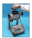
Vial shield shipping cover is replaced with the drawing shield cover.
