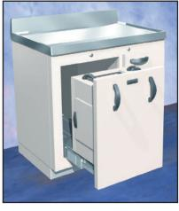
he Generator and Storage Cabinet provides hot lab radiation protection without hampering the elution process. The left drawer accommodates top or side loading generators. In addition to the .5" or 1" lead shielding in front, the drawer has .25" lead shielding on the remaining three sides and bottom. A removable drawer top allows generator replacement. Trap doors on the top and sides of this drawer
