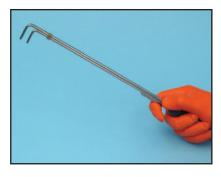
These low-cost tongs are used to handle small radioactive or otherwise dangerous objects up to 1" diameter. The tongs have a 45° v cut groove on each jaw. The compression spring maintains a strong grip on the object until the tension is released by
