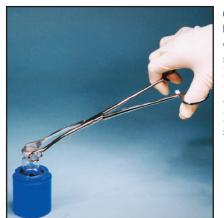
**S**urgical forceps are excellent handling devices for small items in the hot lab. No need to physically touch vials, ampules, etc. Forceps are made of surgical grade steel.
