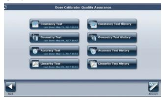
The Atomlab 500 has been designed to make life easier. The extensive selection of quality assurance applications streamlines and simplifies hot lab administration requirements. The system stores and decay corrects multiple reference sources and compares the measured activity to the calculated activity for the daily constancy test.
