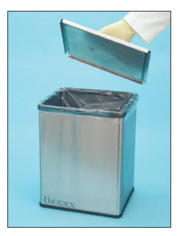
The Shielded Waste Container is a must-have item for any facility that generates low-energy gamma radiation waste. Constructed entirely of 18-gauge stainless steel and lined with .125" lead, this 20-quart container can be placed on the floor or counter. Simply lift off the shielded cover for quick disposal of waste. Plastic liners make it easy to transfer waste to a decay or disposal site once the container is filled.
