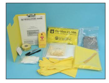
The Emergency Spill Kit is based on suggested contents described in NRC Regulations Guide 10.8, Revision 2: Medical Use Programs, Appendix J: Medical Spill Procedures. Designed to handle minor radioactive spills and routine contamination problems in the lab, it also includes the emergency procedures and forms to document the spill and decontamination clean up.
