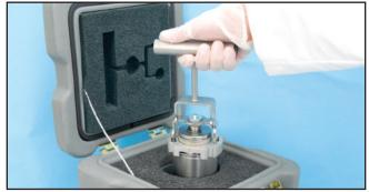
The Vial Shipping System employs a unique Tungsten Vial Shield for use with the Medrad<sup>®</sup> Intego<sup>™</sup> PET Infusion System. Manufactured to Medrad's specifications, the Vial Shield transports a 30 ml Hospira vial.
