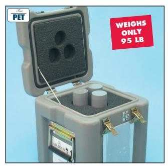
The system meets DOT Yellow II Type A packaging requirements when shipping up to 235 mCi (8.70 GBq) in one pig, and 160 mCi (5.92 GBq) in the second pig and 140 mCi (5.18 GBq) in the third pig, totaling 535 mCi (19.80 GBq) of FDG F-18.
