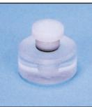
tacle, 1" diameter x .5" thick, has a centered channel to contain 0.2 cc of the nuclide. A nylon screw-plug tightens against an O-ring completing a tight, safe seal. Marker is re-usable or nuclide
