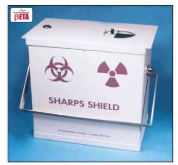
This Sharps Container Shield is a simple way to dispose of used syringes that may be contaminated with low-energy gamma and beta radiation residue. The shield is constructed of steel, lined with .125" lead and .0625" aluminum. The shield-ing combination attenuates gamma radiation, beta radiation and errant bremsstrahlung.
