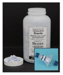
**D**rierite serves as a moisture trap for the air going into the charcoal trap of the Pulmonex Xenon System. Drierite is blue and white when dry and turns pink when it has absorbed maximum moisture. Available in two convenient sizes, Drierite is packaged in an airtight container with a wide-access mouth.
