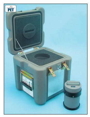
Transport up to a 30 ml vial of PET pharmaceutical in the PET Shipping System. The complete system offers 1.55" lead shielding to accommodate 1.5 curies of FDG F-18 and meets DOT II Type A packaging requirements.
