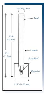
The Pen Point Marker Source contains Co-57 in a ceramic matrix at the end of a 9.26" (23.5 cm) anodized aluminum rod. The pen-shaped rod screws into a brass cap which shields the active point. The Pen Point Marker Source is used in tracing the outlines of anatomical features on a patient. The trace appears almost instantly on the camera display. Contained activity is supplied as a nominal value  $\pm 15\%$ .
