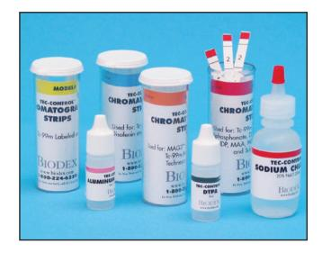
∎ec-Control<sup>™</sup> Chromatography tests the radiochemical purity of specific Tc-99m-labeled radiopharmaceuticals. The accompanying chart shows which strips and solvents are required to perform each individual test. Some solvents must be purchased separately (see Sigma-Aldrich chart) due to hazardous material shipping restrictions.
