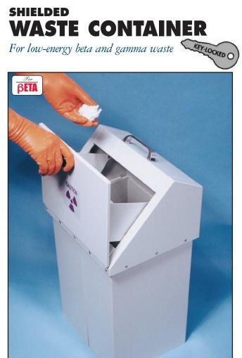
This Shielded Waste Container is used in facilities that generate low-energy beta and gamma radiation waste. The interior of the container is constructed of .063" aluminum and .25" lead. The shielding combination attenuates gamma radiation, beta radiation and errant bremsstrahlung.
