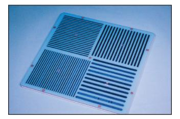
**P**our-quadrant Bar Phantoms offer precise determination of camera intrinsic resolution, collimator spatial resolution, field size and linearity. We offer a range of sizes manufactured to the highest quality standards.
