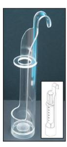
The Syringe Dipper will hold a 60 cc syringe in the correct position in most commercial dose calibrators with  $2.5" \ge 10"$  well chamber interior. The material used will not cause attenuation problems and is very resistant to breaking.
