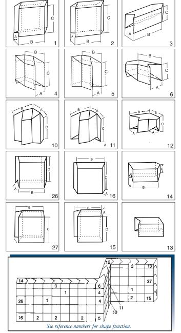
This wall demonstrates the dimensions and alternative positions of all variations of the standard brick wall. The walls should be built with male chevrons directed upwards and to the right, as viewed from the outside of the cell.
